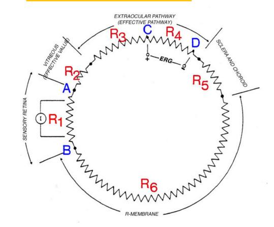
An electrical scheme of the resistances through which currents IA and IB flow when the retina is stimulated with light. The current source I, represents the electrical current that is generated in the retina in response to a light stimulus. Pathway A is the local intra-retinal route of current flow and pathway B is the remote route going from the retina and through the vitreous, lens, cornea, extra-ocular tissues and back to the retina through the sclera, choroid and pigment epithelium.
